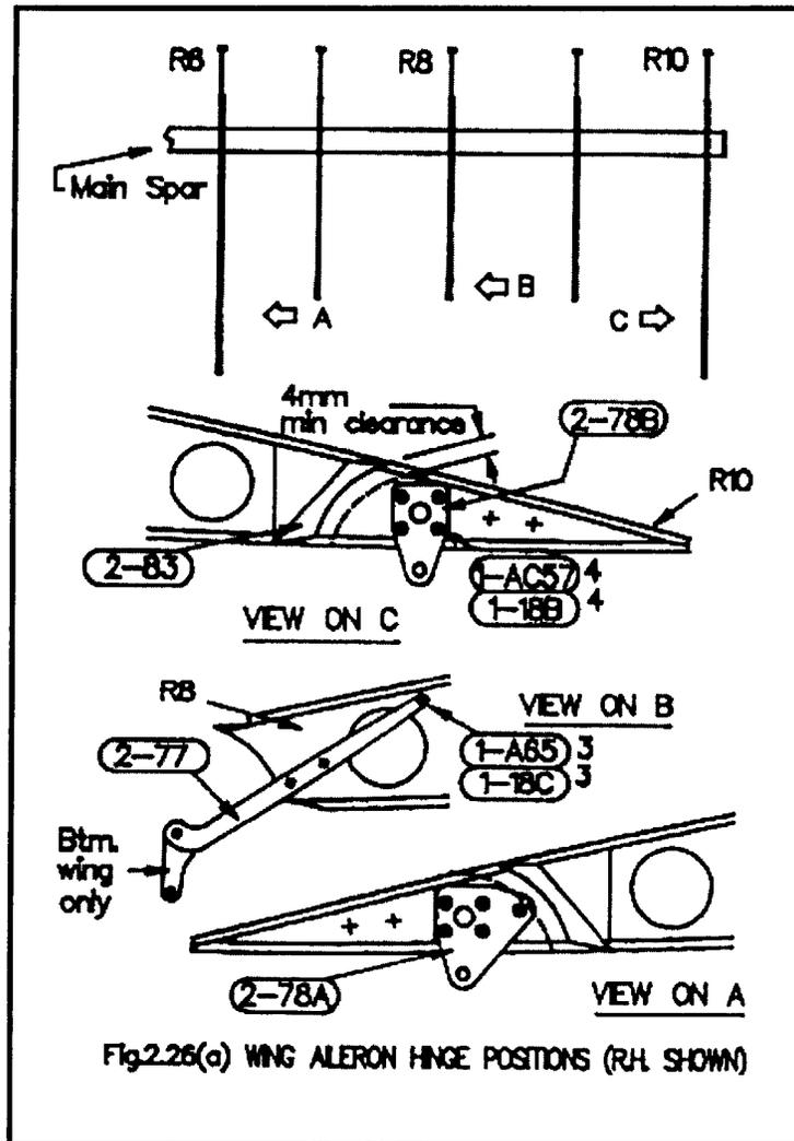
clearance of approximately 4mm. is maintained between the aileron cut-out web and the aileron leading edge sheet.
