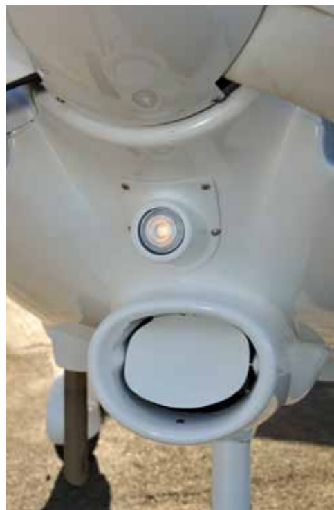
The flight-adjustable cooling air intake flap facilitates rapid warm up on the ground and fine temperature control in the air
