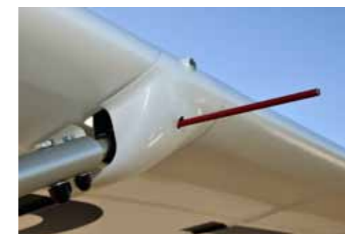
The delight is in the detail: cuffs around the strut mounts are one of many aerodynamic improvements aimed at reducing drag and enhancing performance
