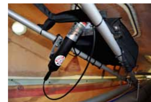
BRS aircraft parachute pack sits on top of the tail boom bracing tubes, ready to be dragged out by the rocket in the foreground
