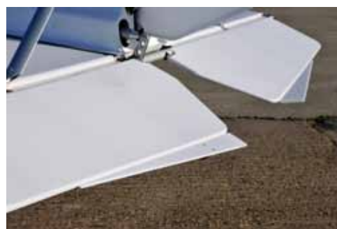
Port elevator tab is an adjustable trim – starboard one a servo tab that lightens control force
