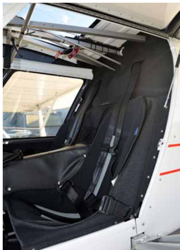
BELOW: carefully contoured and thinly padded fixed seats are designed to be of minimal mass yet offer good comfort
