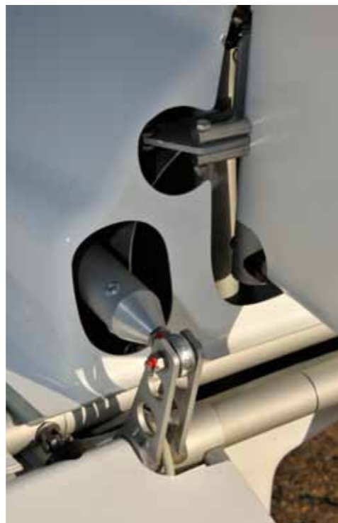
Nicely engineered elevator and rudder controls. Note the large diameter pushrod, designed to prevent buckling under extreme load
