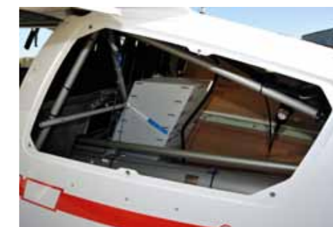
Removing the fuselage hatch reveals the hidden fuel tank and lamp post-sized fuselage boom that carries the structural load (the outer skin just defines the shape and aerodynamic profile)
