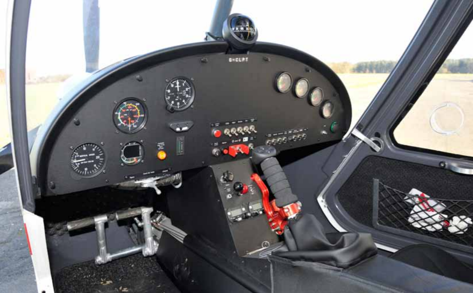
ABOVE: fitted here with the all the basic analogue instruments you need for Day VFR flight, the C42's panel offers loads of space for glass displays and other optional extras
