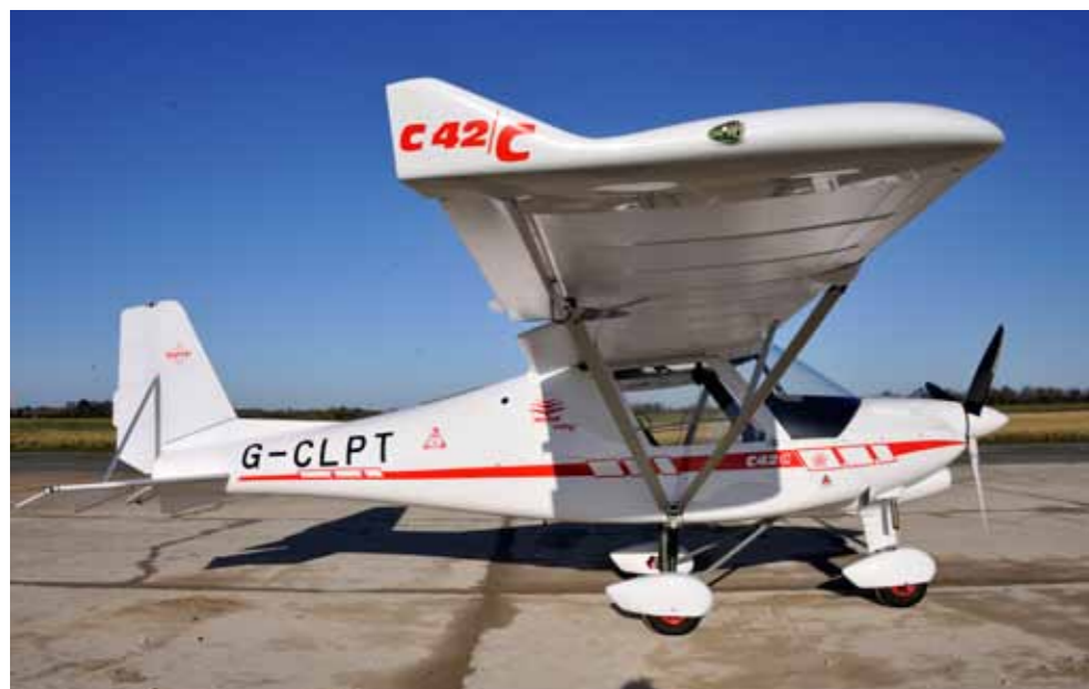
C model improvements include a low-drag aerofoil section and distinctive winglets
